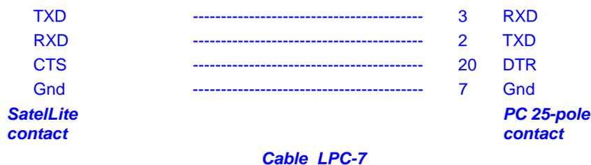
At startup of SatelLite you get a standard setting of the serial inport, which is 9600 baud, 8 bits, 1 stop-bit, no parity. WinSat and WinLog will automatically adjust to this.
